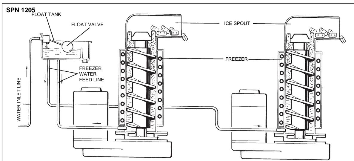
By running the ice maker, i.e. by putting the unit under power, starts the automatic and continuous icemaking process which would not stop until the ice storage bin gets filled-up to the level of the control "eyes" located on the ice chute. As the ice level raises to interrupt the light beam running between the two infrared leds (one or both on model SPN1205), the unit stops after six seconds, with the simultaneous glowing of the **YELLOW LED** signalling the "Full Bin" situation.
