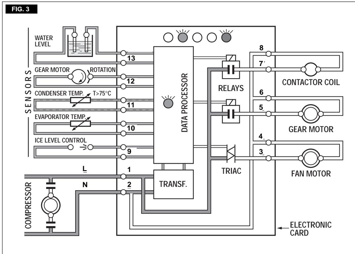
**NOTE.** If, after ten minutes from the compressor start-up, the evaporating temperature has not dropped down to a value lower than  $-1^{\circ}\text{C}$  ( $30^{\circ}\text{F}$ ) the evaporating temperature sensor detects such an abnormal situation and stops consequently the unit operation. In this circumstance, the **5th warning YELLOW LED** will blink.
