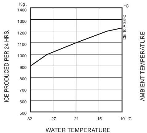
**NOTE.** The daily ice-making capacity is directly related to the condenser air inlet temperature, water temperature and age of the machine.
