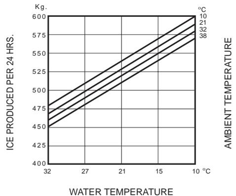
**NOTE.** The daily ice-making capacity is directly related to the condenser air inlet temperature, water temperature and age of the machine.
