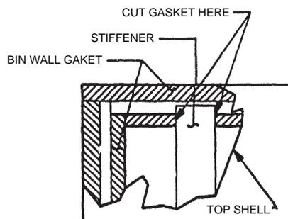
**NOTE.** Bin wall gasket must be cut to clear the stiffener ends as shown on drawing. Do not put any stiffeners crossing the ice drop opening.
