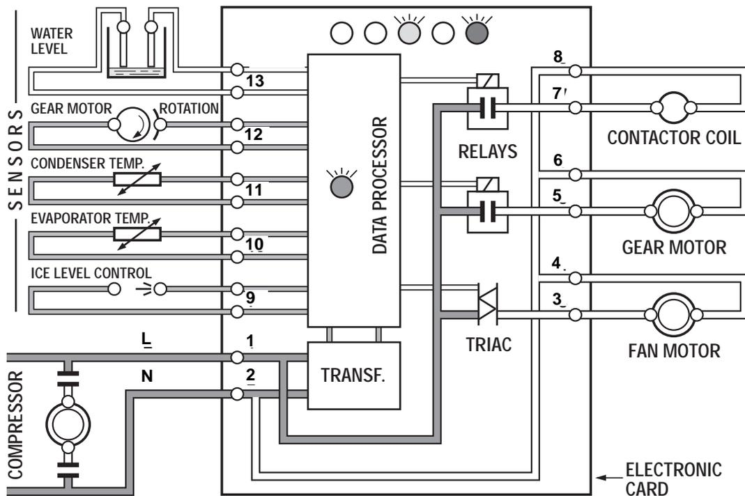
This will cause a gradual decrease of the water level in the float reservoir and as soon as the level gets below the two vertical metal pins, the flaker stops to operate and the **YELLOW warning LED** will glow to signal the shortage of water (Fig. 4)
